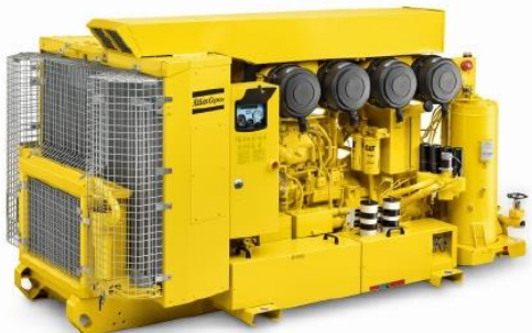
Drill Air™ Open Unit Wagon-mounted two-stage, oil-injected, asymmetrical rotary screw compressors, 25-30 bar (365-435 psig)
