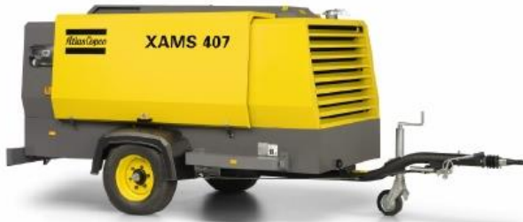
Size 2 LP Single axle, oil-injected, rotary screw portable compressors, 8.6-14 bar (125-200 psig)
