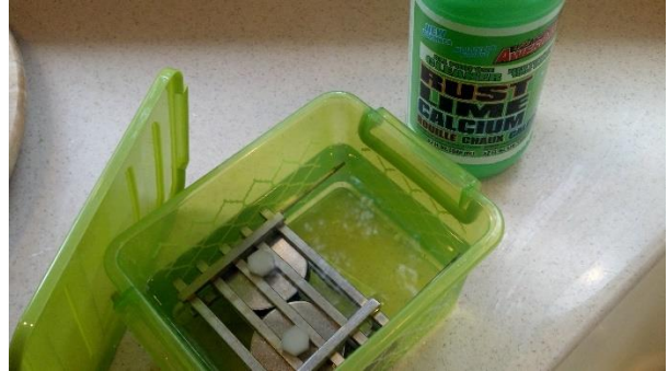
Soak array in cleaning solution
